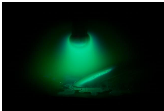
Fig. 13. Metal drop at the filler wire tip
