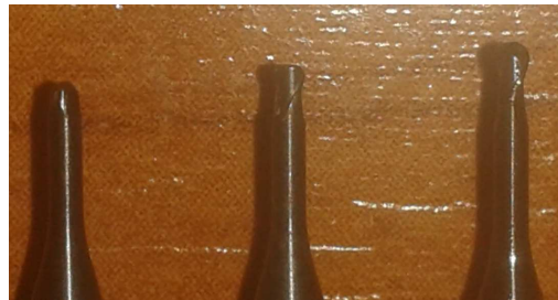
Fig.7 : Tool after wave form, after cycloid form, unworn tool
