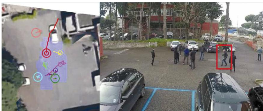
Figure 1: Feature level fusion of multispectral (EO, IR) views which highlights mismatches and 'invisible' human shapes.
