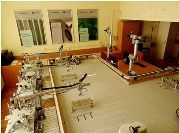
Fig. 3. Partial view of the Smart Factory at MTA SZTAKI, showing 3 of the 4 workstations (left), one of the mobile robots (center), and the two manipulators (right)
