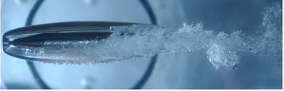
Figure 2.1: Supercavitation water tunnel test at Saint Anthony Falls Laboratory (UMN).
