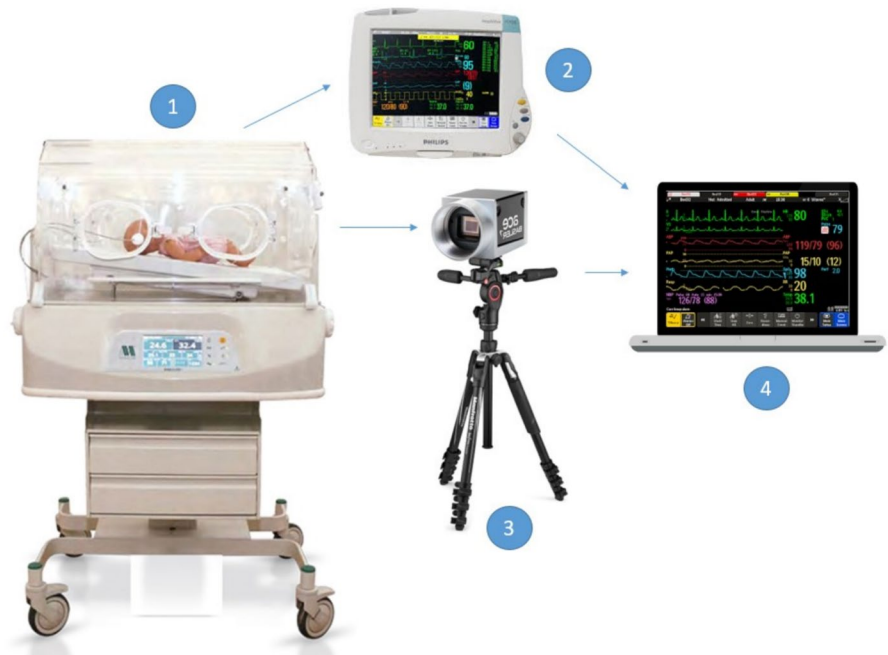
Fig. 1 In the experimental setup the neonatal infant in NICU (1) was monitored with a Basler acA2040-55uc RGB camera (3). At the same time, physiological signals were received from the Philips IntelliVue MP20/MP50 monitors (2). The wave and rate data from the monitors and the video images from the camera were saved in sync to a laptop (4)
