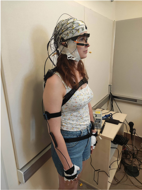
FIGURE 2 Sensors used in the BG. The participants were equipped with high-density EEG, wearable eye tracker, inertial motion capture system, and headset microphone.
