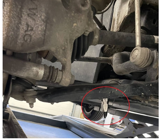
Fig. 4. Three axis accelerometer used to collect vibration data.
