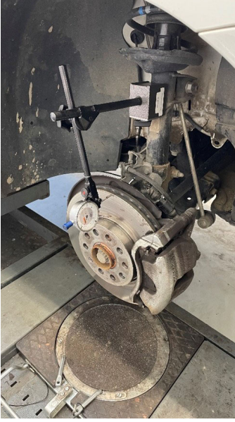
Fig. 2. Brake disc runout measurement with dial gauge.
