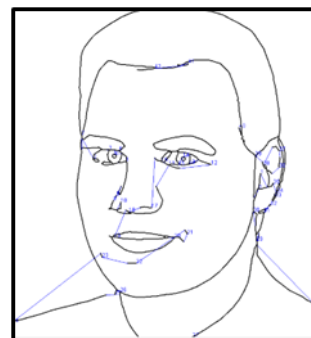
Figure 16. Visualizing the sequencing algorithm. The black colour indicates the actual drawing, and the blue colour shows the paths travelled in the air by the robot [28].
