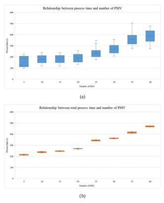
Fig. 7 The process time results with the number of PMVs up to 40, (a) Process time, (b) Total process time
