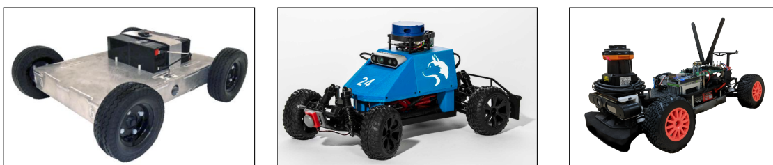
Figure 1.1: Different small-scale vehicle platform used in research and the industry: SuperDroid 1 (left), MuSHR 2 (center), F1TENTH 3 (right).
