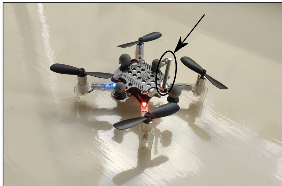
Figure 7.8: Crazyflie 2.1 quadcopter with reflective markers and a bolt (marked with an arrow) used as additional disturbance.
