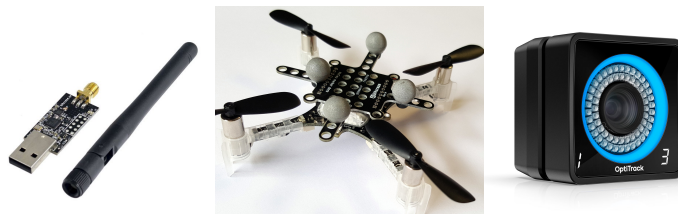
Figure 7.2: The Crazyradio PA, Crazyflie 2.1 with motion capture markers, and an OptiTrack Prime 13 camera.
