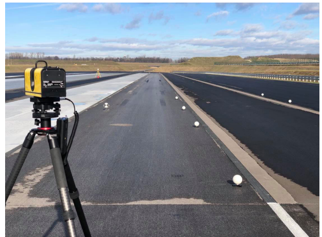
FIGURE 2. TLS survey-surphaser 400 laser scanner (aquaplaning basin).
