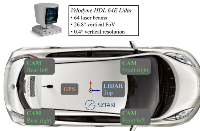
Figure 1: SZTAKICar: The measurement platform.
