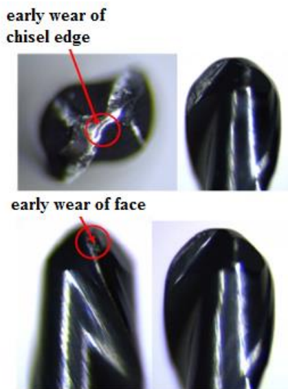
Fig. 7. Tool wear at 40% of the tool life
