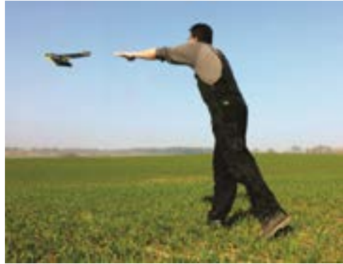
Figure 1 Launch of a senseFly eBee aircraft
