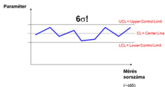
4. Diagram: Statistical process control during the extreme load
