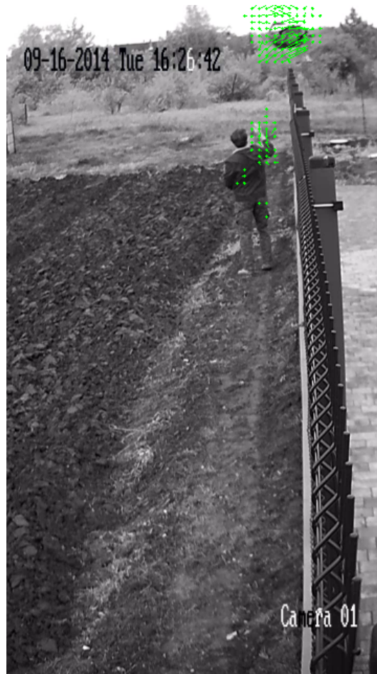
Fig. 2. Detected optical flow on the foreground of the image. Only flow vectors with length greater than 1 are shown.
