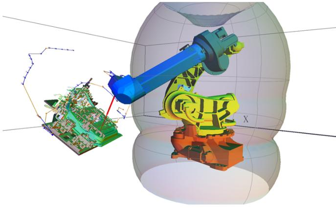
Figure 1: RLW robot welding a car front door, positioned in a fixture. The blue sections of the indicated scanner path represent the movement of the robot while welding, while yellow sections denote idle movement.
