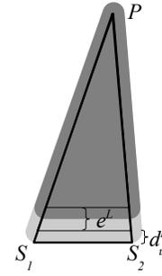
Figure 5: Mesh model of the laser beam for welding the linear stitch  $\overline{S_1S_2}$  from robot position  $P$ . The approach results in the light gray collision zone for fixture, and the dark gray collision zone for both the fixture and the workpiece.
