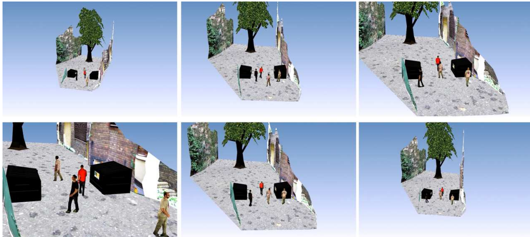
Figure 23: Object tracking and reconstruction results. Upper left: raw point cloud; lower left: segmented and separated objects; upper right: trajectories from upper view; lower right: reconstructed environment, the studio objects placed to the original positions.
