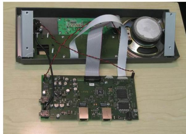
**Figure 1. Audio equipment assembly for testing, where 2D pictures are not enough for completeness inspection**
