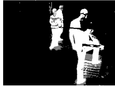
(a) Shadows may corrupt foreground detection even in carefully chosen color space. Foreground mask (right) for an input frame (left) is shown. A number of false positives are introduced due to corrupted foreground mask.
