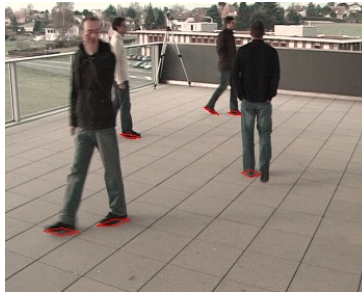
(c) Candidate pixels are clustered, clusters are modeled with ellipses (ellipses are visualized with lozenges).
