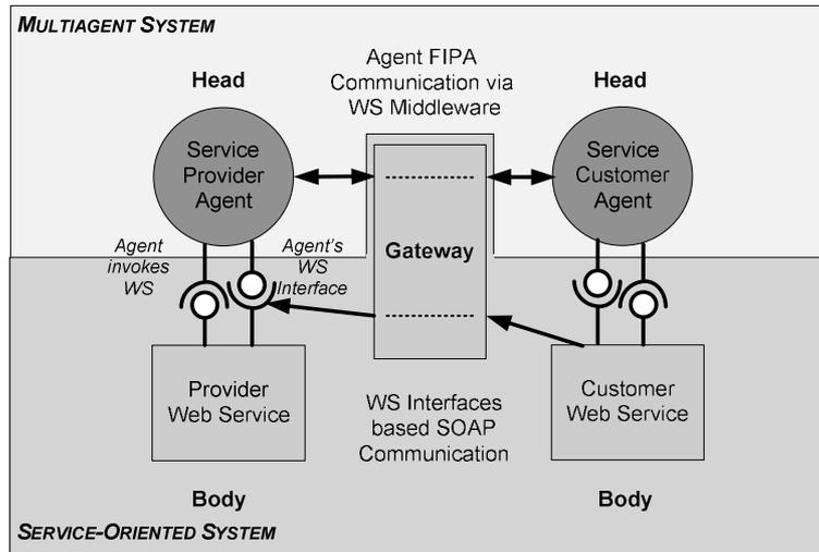
**Fig. 1.** Head Body Architecture
