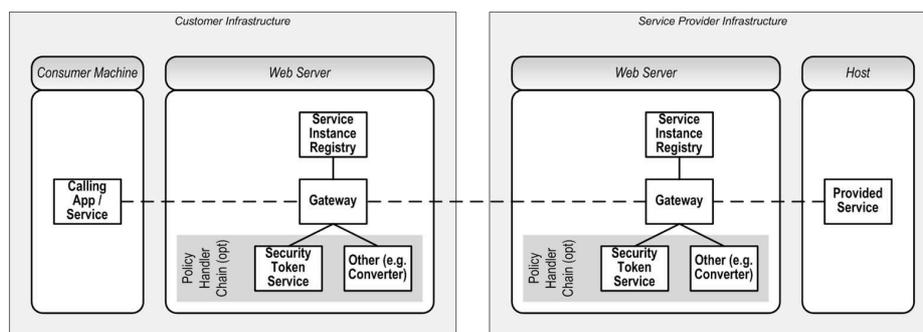
**Fig. 2.** Sample deployment of the Gateway infrastructure
